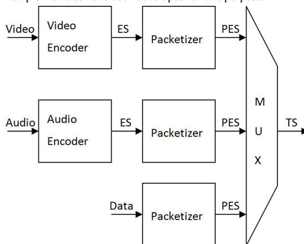
Figure 1. A program multiplexed on a transport stream.
