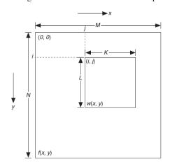
Assume that the origin of the image f is at the top left corner. Correlation is the process of moving the template or sub-image w around the image area and computing the value C in that area. This involves multiplying each pixel in the template by the image pixel that it overlaps and then summing the results over all the pixels of the template. The maximum value of C indicates the position, where w best matches f. Correlation is not accurate at the borders of the image.
