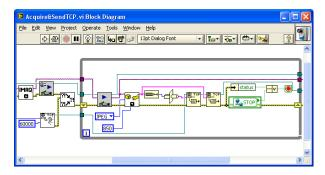
2. Host part, which implement the analyzing of received image data via pattern matching algorithm and then send the results to mouse move controlling subVI's. It is possible to move mouse via face moving, left click and double click.
