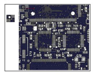
The traditional methods have no learning phase; the template is simply compared to every possible location in the image via a 2D correlation. This is very computationally intensive and involves many redundant calculations. Below is an example of a printed circuit board and template. After performing the correlation at every point in the image, two matches were found.
