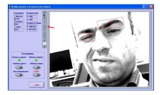
You can change some parameters of image being acquired, as it's brightness, contrast and gamma, then you have to learn and set templates for mouse click and mouse move, you can do auto calibration of template position on an image, then start control mouse by moving your head.
