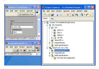
1. Real-Time part, which is sending acquired image via TCP/IP to the host computer. The program is compressing image data to JPG format before send to be able send more data in unit time. Below is the block diagram of that program.
