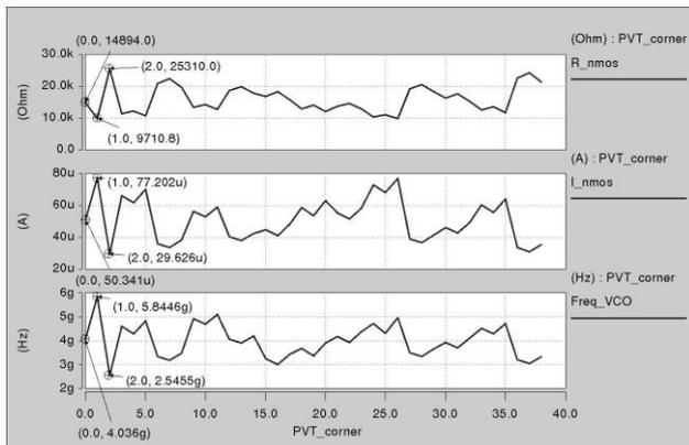
Fig. 9. Detection NMOS resistance calibration effect for all PVT corners.
