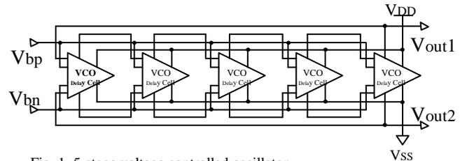
Fig. 1. 5-stage voltage controlled oscillator
