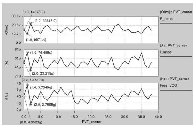
Fig. 10. Detection PMOS resistance calibration effect for all PVT corners.
