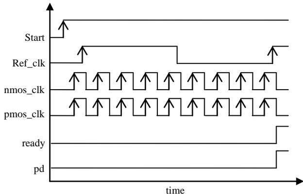
Fig. 7. Logic block simplified timing diagram.
