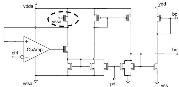
Fig. 5. VCO circuit biasing (PMOS structure).
