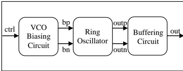
Fig. 2. VCO circuit block-diagram.
