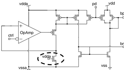
Fig. 3. VCO biasing circuit (NMOS structure).
