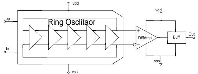
Fig. 4. VCO ring oscillator and buffering circuit.
