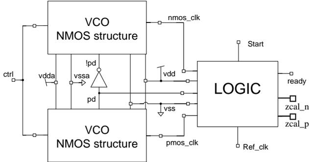
Fig. 6. PMOS and NMOS resistance calibration circuit.
