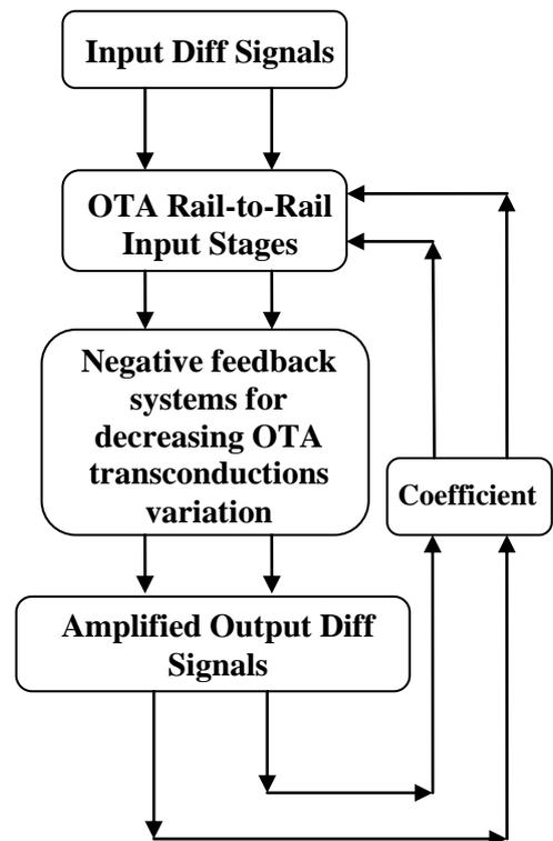
Fig.6. Block diagram of proposed method with negative feedback
