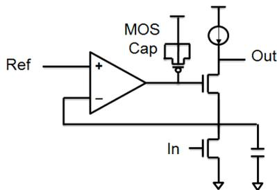
Fig.5. Using MOS capacitor for booster fine-tunes.
