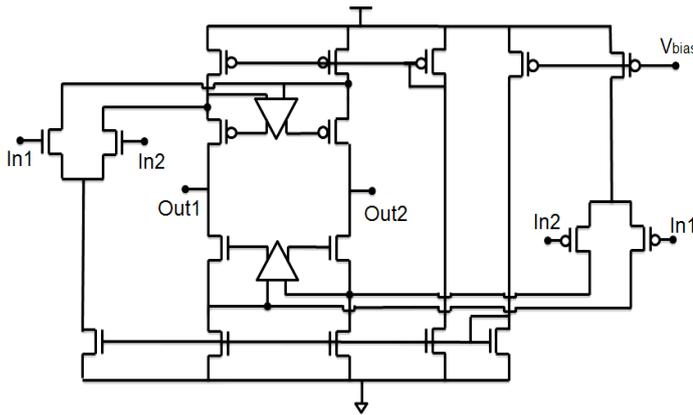
Fig.4. Circuit structure GB OTA with Rail-to-Rail inputs
