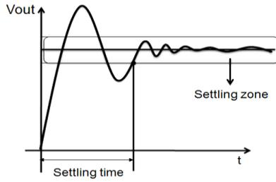
Fig.3. Settling time calculation
