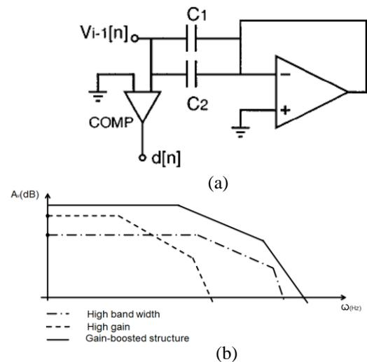
Fig.2. (a) Gain boosted OTA Using In The  $i^{th}$  Stage Of A 1-bit/stage Pipeline ADC
