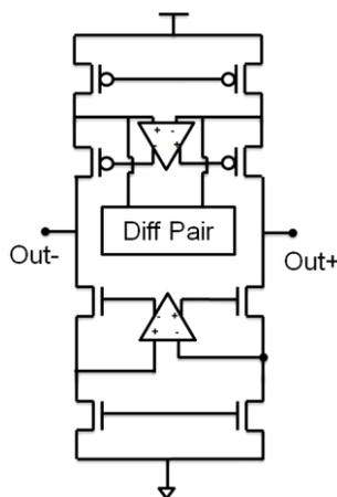
Fig.1. Gain-Boosting Technique
