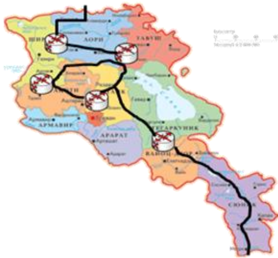
the basic transmission network, based on fiber optic equipment
