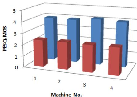
Figure 6: Comparison of PESQ-MOS values for wired (blue columns) and wireless (red columns) network simulations
