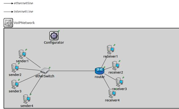
Figure 2: Network for wired simulation scenario
