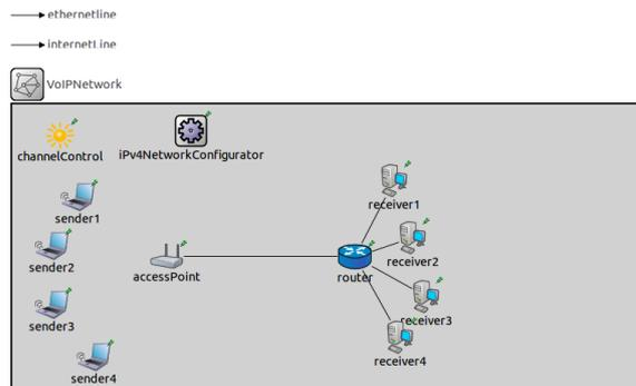
Figure 3: Network for wireless simulation scenario
