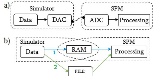
Picture 2. Simulator-SPM data transfer, a) analog, b) digital
