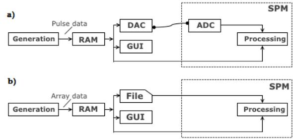
Picture 1. Using ways in a) echo mode, b) pack mode
