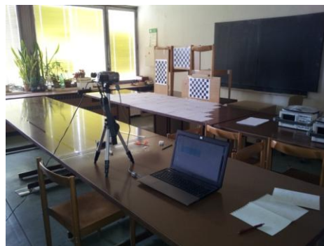
Figure 9. The stereo pair configuration
