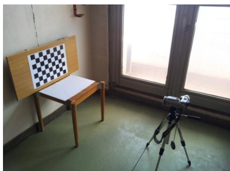
Figure 8. The camera calibration
