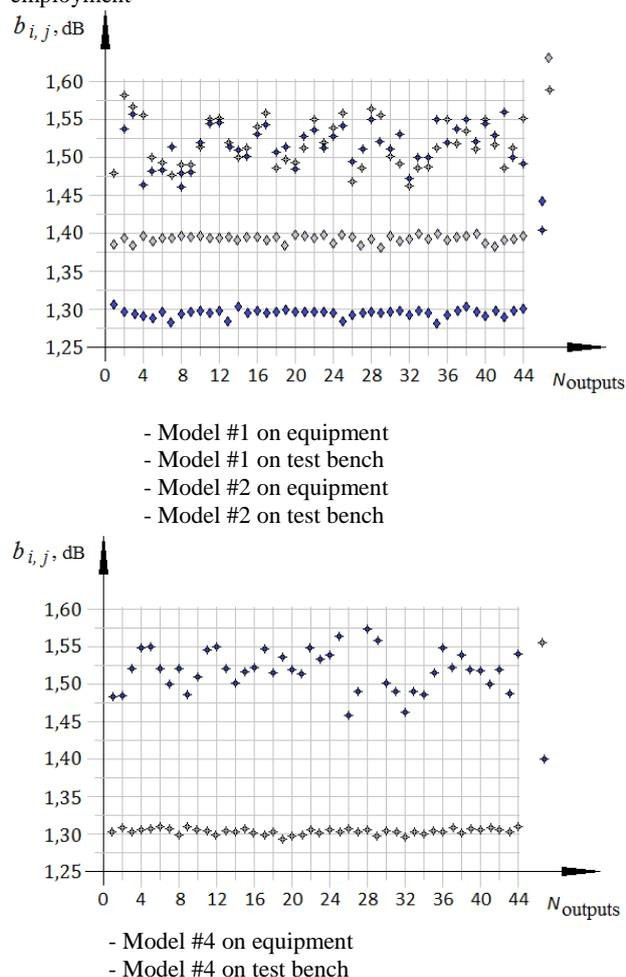
Fig. 6. Transmission coefficient determination (with splitting) results for the OSCD models #1, #2 and #4 with test bench employment: a) – for OSCD models #1 and #2; b) – for OSCD model #4
