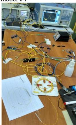
Fig. 7. Loss and transmission coefficients measurement process for the OSCD models #1 within test bench equipment
