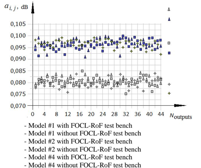
Fig. 5. Loss coefficient determination (with splitting) results for the OSCD models #1, #2 and #4: a) – with frame-controller employment; b) – with test bench emitter employment
