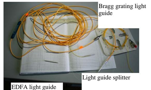
Fig. 4. Long-haul OSCD model scheme #4 (models #3, #5 and #6 externally look similar)
