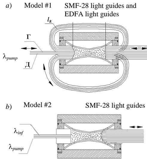
Fig. 1. The OSCD models schemes: a) – the model provides splitting function  $1 \times 44$ , recommended for AA use; the number of output light guides can be increased if necessary;  $\lambda_{inf}$  – informational signal emission wavelength and  $\lambda_{pump}$  – pump emission wavelength (necessary for EDFA light guides, equal to 980 nm); b) - the model provides splitting function  $1 \times 44$ , recommended for AA fixed lobe positioning
