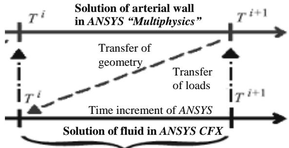
Fig. 5. The diagram of interaction between modules ANSYS CFX and ANSYS “Multiphysics”.
