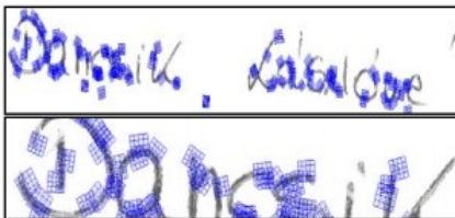
Figure 5. Feature extraction using the SIFT algorithm and the magnified image displayed for greater clarity [15]
