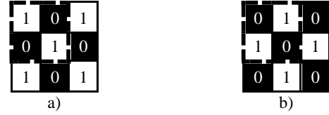
Figure 3. Masks of the convolutional filter, the use of which is "equivalent" to the operation CHB0: a) 101010101, b) 010101010
