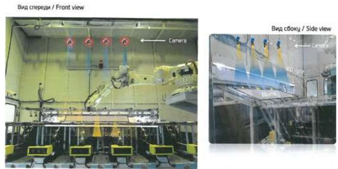
Fig.8. Location of cameras on the production line
