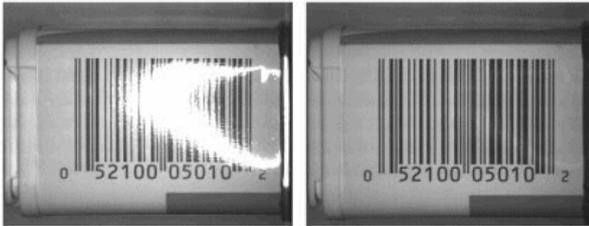
Fig.3. Reflection of light from a surface, the importance of choosing the right lighting
