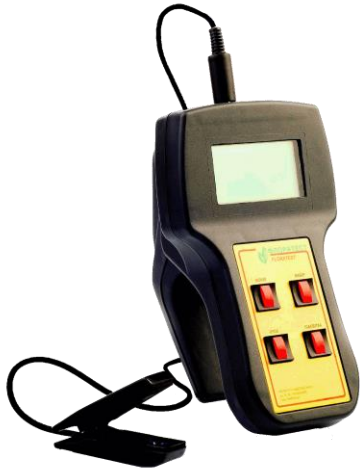
Fig. 1. Computer device for express diagnostics of plant state "Floratest"
